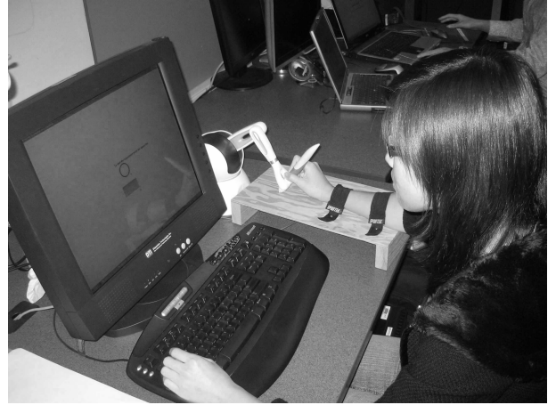
Fig. 1. Experimental setup for the study on the perception of force magnitude
