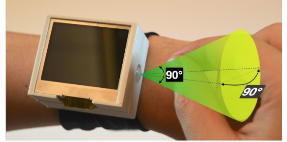
Figure 4. A smartwatch prototype augmented with Pyro.
