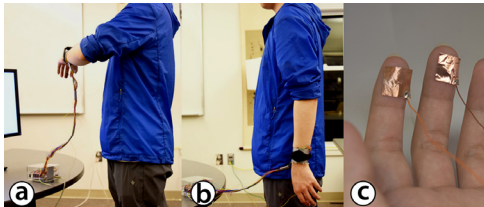
Figure 9. Study setup. (a) hand-up condition; (b) hand-down condition; and (c) capacitive sensors.
